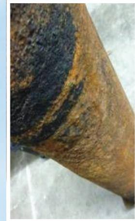
3 Views of the corroded sample from well riser pipe.
